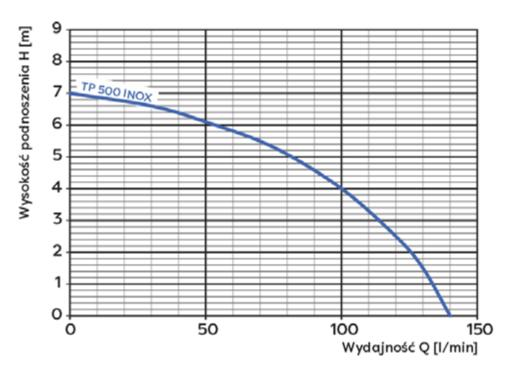
Parameter charts [Rys. Y: Head max H [m], X: Capacity Q [I/min]]
